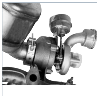
Automotive: Turbocharger – catalytic converter connection
